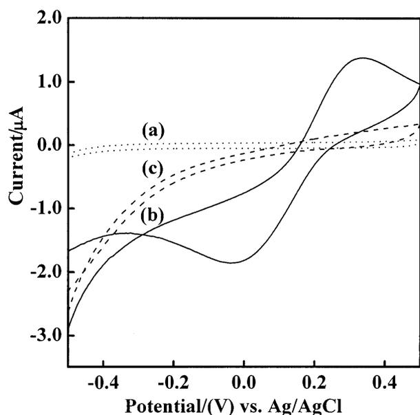
**Figure 2.** Cyclic voltammograms at a bare Au electrode. (a) Blank, (b) 0.5 mM potassium ferrocyanide, (c) 0.5 mM potassium ferrocyanide + 30  $\mu\text{g/ml}$  SBA. Measurements using scan rate 50 mV/s in 0.1 M phosphate buffer (pH 7.0).
