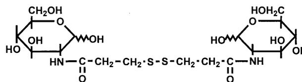
**Figure 1.** Modifier obtained by reaction between galactosamine and DTSSP.
