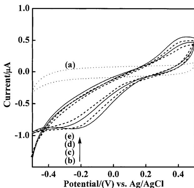
**Figure 3.** Cyclic voltammograms at galactosamine-modified electrode. (a) Blank, (b) 0.5 mM potassium ferrocyanide or 0.5 mM potassium ferrocyanide + 30  $\mu\text{g/ml}$  Con A, (c) 0.5 mM potassium ferrocyanide + 15  $\mu\text{g/ml}$  SBA, (d) 0.5 mM potassium ferrocyanide + 30  $\mu\text{g/ml}$  SBA, (e) 0.5 mM potassium ferrocyanide + 45  $\mu\text{g/ml}$  SBA. Measurements using scan rate 50 mV/s in 0.1 M phosphate buffer (pH 7.0).
